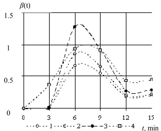
**Fig. 2.** Parameter  $\beta_\nu$  versus time  $t = 3m$  at  $\nu$  of (1) 1750, (2) 2000, (3) 2500, and (4) 3000 rpm.
