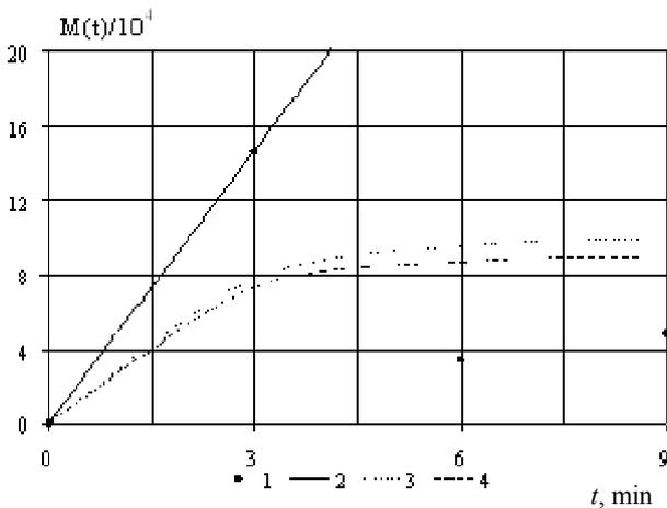
**Fig. 3.** Number of bubbles versus time  $t$  in the rotor-stator processing of a protein solution for (1) experimental data and  $\beta_{2500}$  of (2) 0.0050, (3) 0.4929, and (4) 0.5476 1/min.
