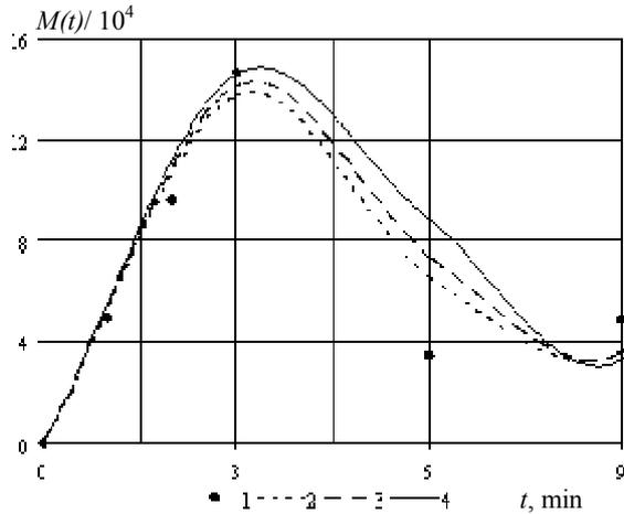
**Fig. 6.** Number of bubbles versus time  $t$  in the rotor-stator processing of a protein solution at  $\beta(t) = \bar{\beta}$  for (1) experimental data, (2)  $A = 7.50$ ,  $B = 0.01$ ,  $a = 6.90$ ,  $b = 2.10$ , (3)  $A = 7.20$ ,  $B = 0.01$ ,  $a = 7.00$ ,  $b = 2.00$ , and (4)  $A = 6.90$ ,  $B = 0.01$ ,  $a = 7.10$ ,  $b = 1.80$ .
