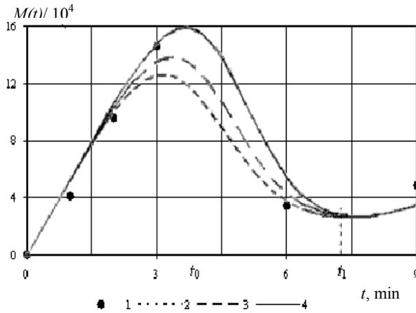
**Fig. 5.** Number of bubbles versus time  $t$  in the rotor-stator processing of a protein solution for (1) experimental data, (2)  $A = 7.50, B = 0.01, a = 6.90, b = 2.10$ , (3)  $A = 7.20, B = 0.01, a = 7.00, b = 2.00$ , and (4)  $A = 6.90, B = 0.01, a = 7.10, b = 1.80$ .
