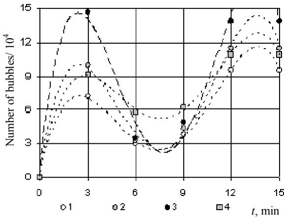
**Fig. 1.** Number of bubbles per unit volume at time moments  $t = 3m$ ,  $m = 1, 2, 3, 4, 5$  at  $\nu$  of (1) 1750, (2) 2000, (3) 2500, and (4) 3000 rpm.
