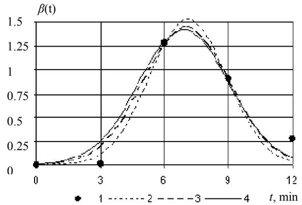
**Fig. 4.** Time function  $\beta(t)$  calculated (1) from experimental data and at (2)  $A = 7.50, B = 0.01, a = 6.90, b = 2.10$ , (3)  $A = 7.20, B = 0.01, a = 7.00, b = 2.00$ , and (4)  $A = 6.90, B = 0.01, a = 7.10, b = 1.80$ .
