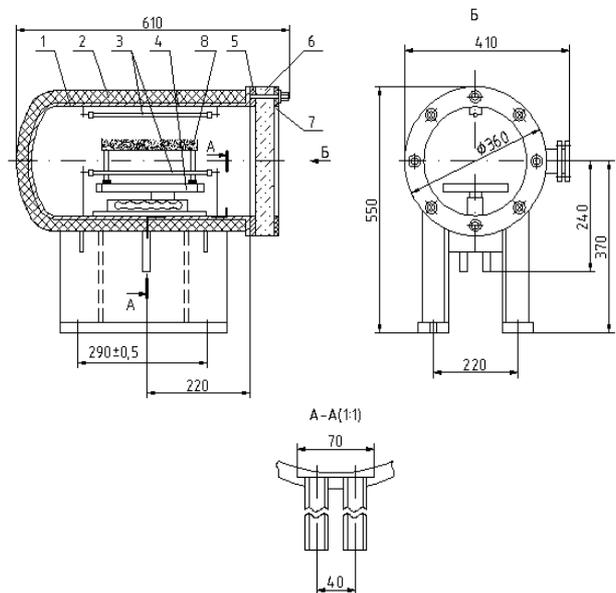
**Fig. 2.** Drying chamber: (1) body, (2) heat insulation, (3) heaters, (4) balance, (5) vacuum-tight rubber, (6) organic glass, (7) sealing ring, and (8) product.
