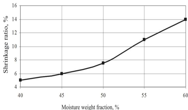
**Fig. 8.** Shrinkage ratio of cheeses as a function of moisture weight fraction.
