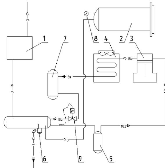
**Fig. 1.** Schematic of the experimental vacuum drier: (1) vacuum pump, (2) vacuum drying chamber, (3) compressor, (4) condenser, (5) liquid separator, (6) desublimator, (7) receiver, (8) vacuum gage, and (9) thermal expansion valve.
