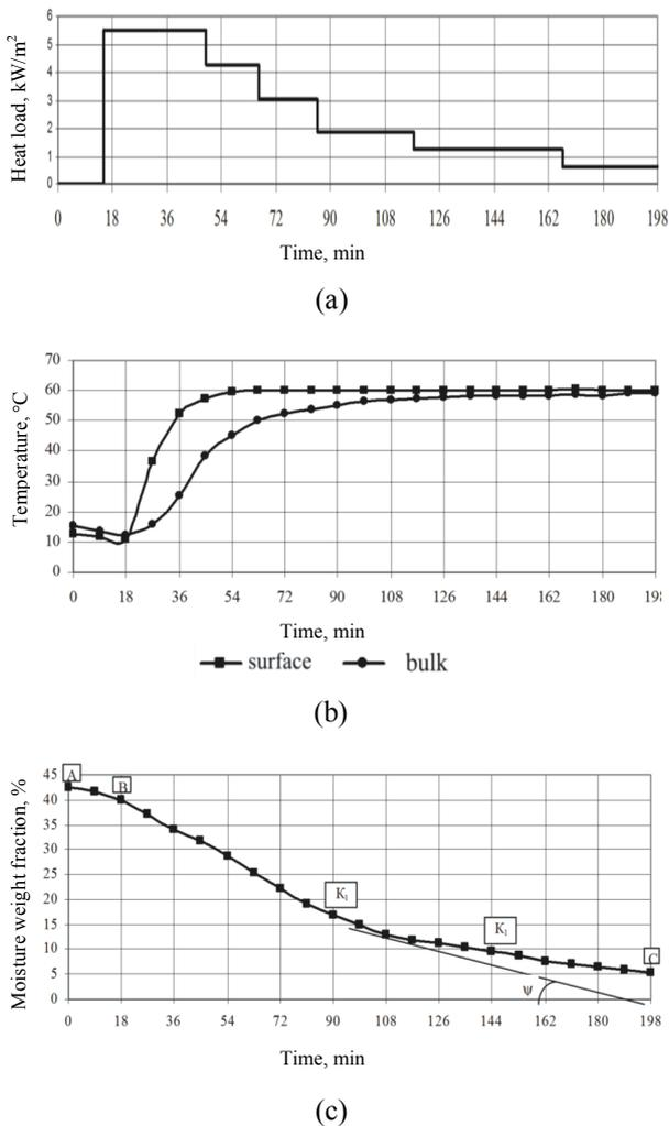
**Fig. 5.** Drying curves for Shveitsarskii cheese: (a) heat load, (b) surface and bulk temperatures, and (c) moisture weight fraction. Drying conditions:  $t = 60^{\circ}\text{C}$ ,  $q = 5.52 \text{ kW/m}^2$ ,  $P = 2\text{--}3 \text{ kPa}$ , and  $h = 10 \text{ mm}$ .
