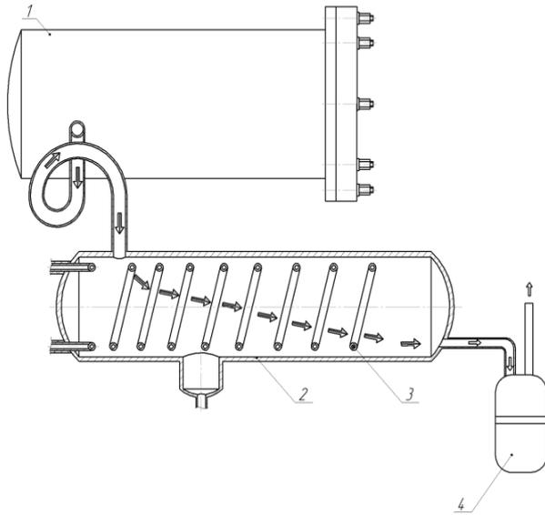
**Fig. 3.** Schematic of the desublimator: (1) vacuum chamber, (2) desublimator, (3) evaporator coil, and (4) vacuum pump.
