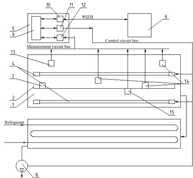
**Fig. 4.** Block diagram of the experimental bench: (1) vacuum chamber, (2) pan, (3) material being dried, (4) IR heaters, (5) interface block, (6) PC, (7) condenser, (8) vacuum pump, (9) microcontroller, (10) PC interface, (11) executor control unit, (12) analog-to-digital converter, (13) pressure sensor, (14) temperature sensor, and (15) load cell.
