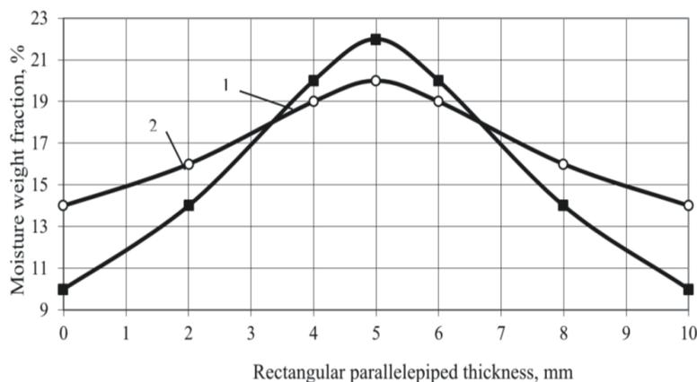
**Fig. 10.** Moisture content profiles along the thickness of (1) cracky and (2) noncracky cheese beds.
