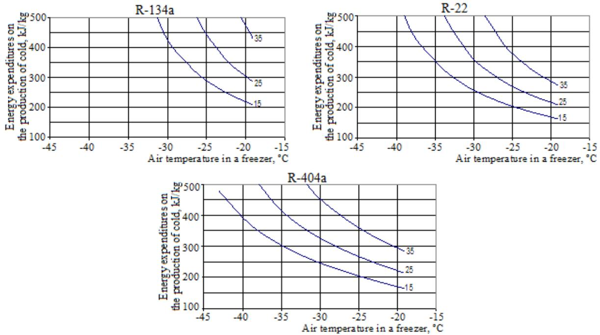
**Fig. 7.** Energy expenditures (kJ/kg) on the driver of a one-stage refrigerating machine for the freezing of a kilogram of Pamyat’ Lisavenko blackcurrant berries from the temperature of 10°C to the temperature of –18°C depending on the air temperature in a fast freezer and the ambient air temperature.
