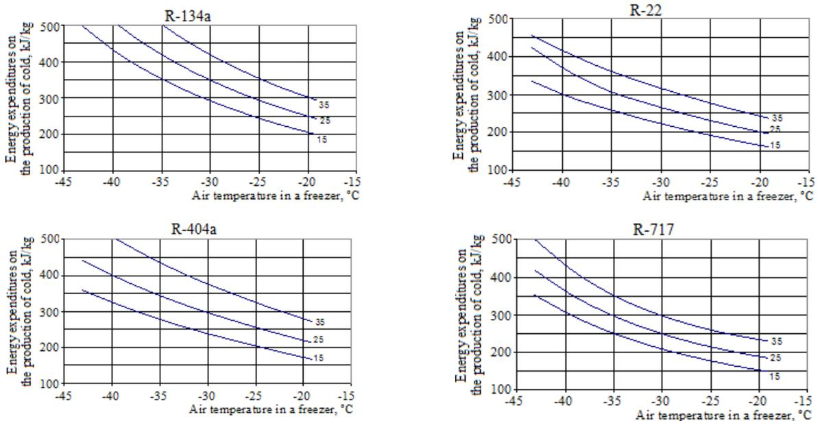
**Fig. 8.** Energy expenditure (kJ/kg) on the driver of a two-stage refrigerating machine for the freezing of a kilogram of Pamyat’ Lisavenko blackcurrant berries from the temperature of 10°C to the temperature of –18°C depending on the air temperature in a fast freezer and the ambient air temperature.
