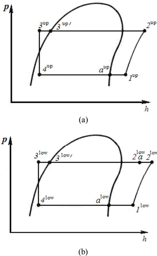
**Fig. 2.** Theoretical cycle of a two-cascade refrigerating machine: (a) upper (high-temperature) cascade branch, (b) lower (low-temperature) cascade branch.
