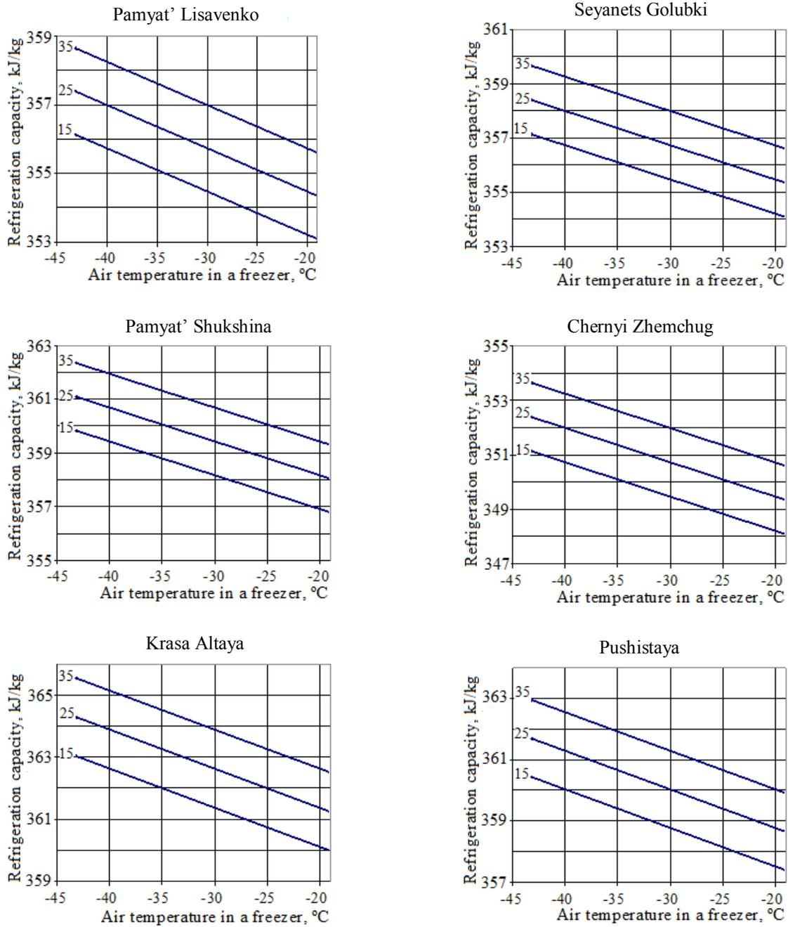
**Fig. 6.** Required refrigeration capacity (kJ/kg) of a refrigerating machine for the freezing of a kilogram of blackcurrant berries from the temperature of 10°C to the temperature of -18°C depending on the air temperature in a fast freezer and the ambient air temperature.
