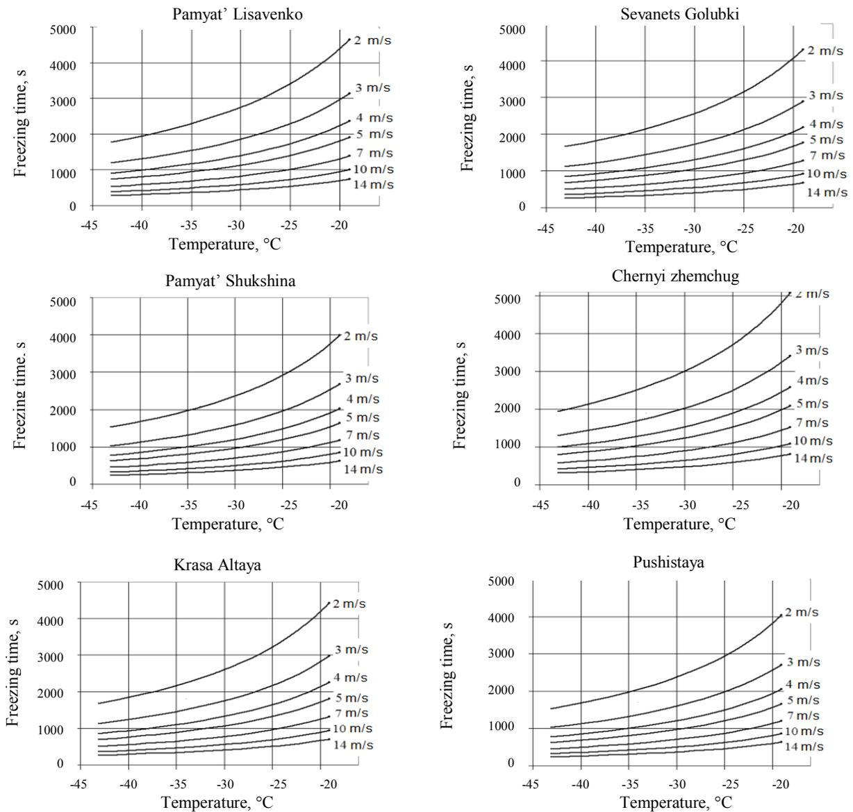
**Fig. 4.** Freezing time versus temperature for the freezing of the studied varieties of blackcurrant berries from the initial temperature of 10°C to the temperature of -18°C in a fluidized-bed fast freezer at different air velocities.
