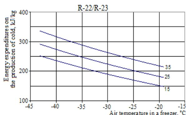
**Fig. 9.** Energy expenditures (kJ/kg) on the driver of a cascade refrigerating machine with freons R-23 and R-22 in the lower and upper cascade branches, respectively, for the freezing of a kilogram of Pamyat' Lisavenko blackcurrant berries from the temperature of  $10^{\circ}\text{C}$  to the temperature of  $-18^{\circ}\text{C}$  depending on the air temperature in a fast freezer and the ambient air temperature.
