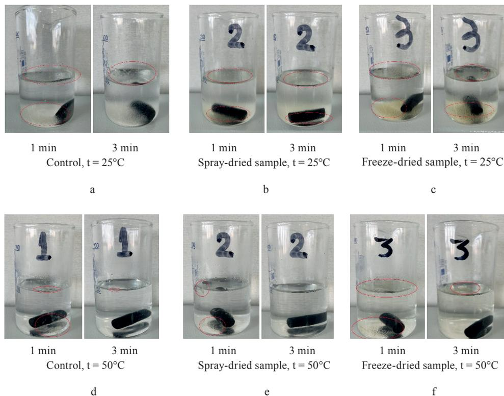
**Figure 1** Dissolution of gelatin samples at 25 and 50°C for 1–3 min
