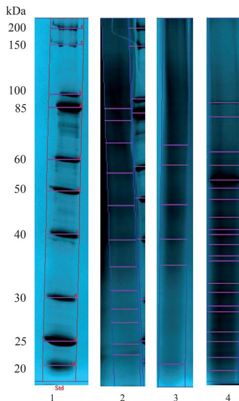
**Figure 4** Electropherogram of the molecular weight distribution of gelatin samples (1 – marker; 2 – control, 3 – spray-dried sample, 4 – freeze-dried sample)
