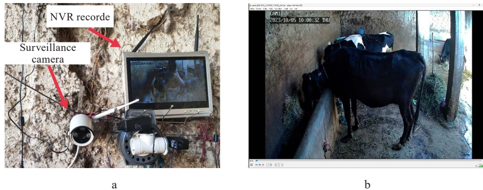
Figure 4 Surveillance camera system components (a) and a screenshot from a recorded video file (b)
