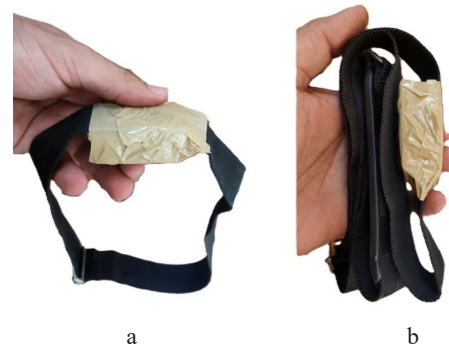
Figure 2 The data collection device attached to an adjustable neck-mounted collar (a) and its length (b)
