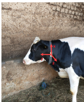
Figure 5 The three-axis neck-mounted accelerometer-based collar
