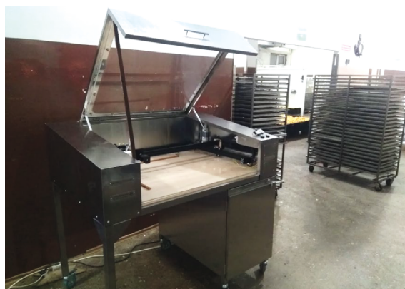
Figure 3 A commercial unit for low-temperature plasma treatment based at Kuban State Technological University
