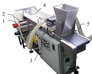
Figure 4 An industrial machine for low-temperature plasma treatment of foods for sterilization [47]: 1 – a discharge chamber, 2 – an electrode unit, 3 – a control panel, 4 – an ozonation chamber, 5 – a belt conveyor
