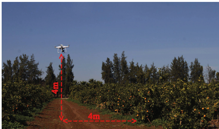
Figure 3 Phantom 4 (P4M) UAV imaging: distance from the tree is 4 m; altitude above ground level is 4 m
