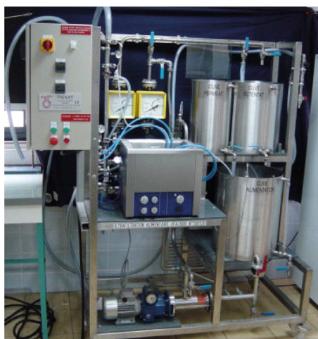
Figure 6 An industrial ultrasonic treatment apparatus for food sterilization [67]
