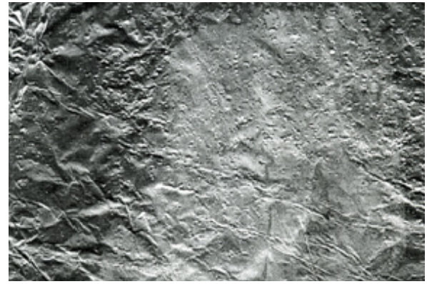
Figure 3 Foil screen deformed by ultrasonic treatment. Processing time – 20 s, distance from the surface of the emitter – 150 mm
