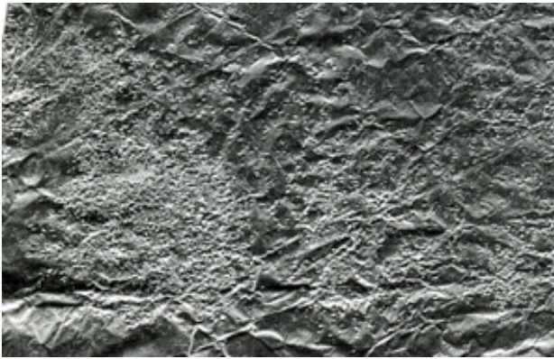
Figure 2 Foil screen deformed by ultrasonic treatment. Processing time – 20 s, distance from the surface of the emitter – 30 mm
