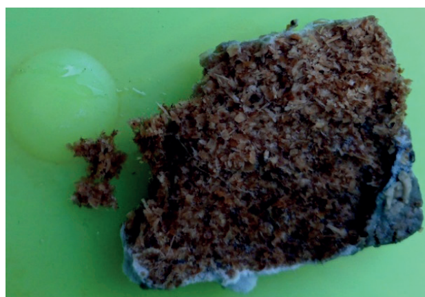
Figure 4 Wood plastic fragment with signs of splitting, swelling, marginal and longitudinal fragmentation
