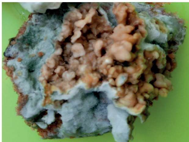
Figure 5 Fragment of plant plastics from wheat husk (without adhesives) with signs of mold growth
