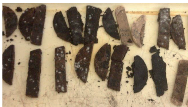
Figure 3 Plant plastic from millet husk, plant plastic from wheat husk, and wood plastic kept in active soil for 21 days (all plastics are made without adhesives)
