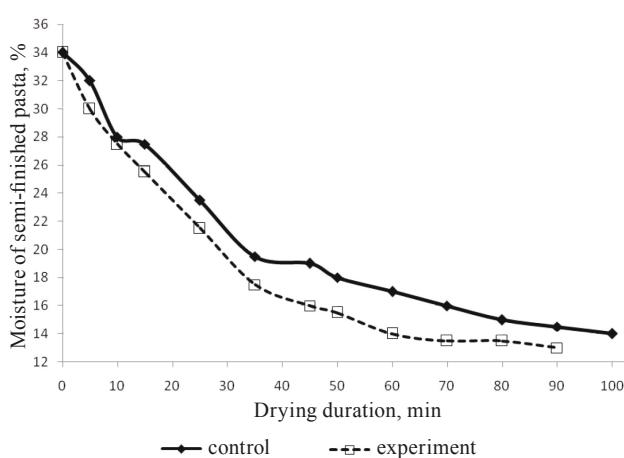
Fig. 3. Drying curves for semi-finished pasta.
