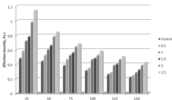
**Fig. 3. The dependence of the effective viscosity on the shear rate in the fermented milk product with different portions of arabinogalactan:**
