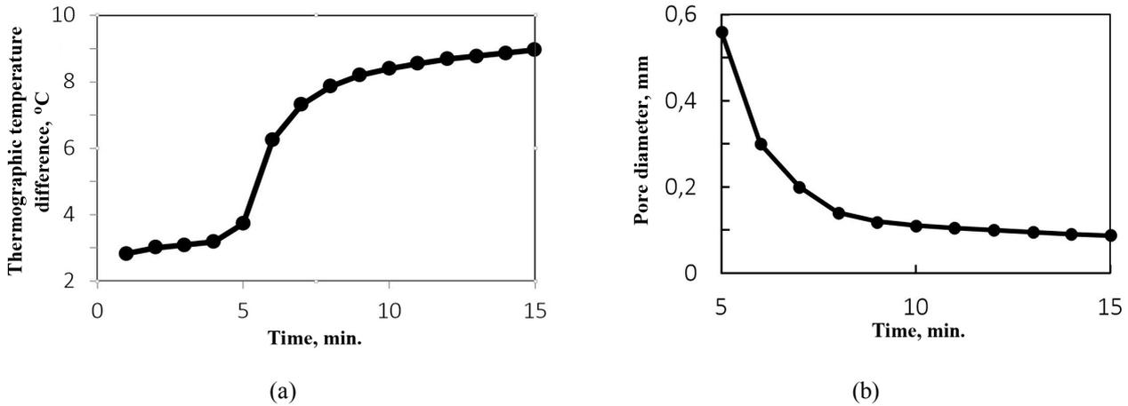
**Fig. 5.** A thermogram of reconstituted skim milk rennet coagulation (a) and (b) estimation of mean pore diameter in this process.
