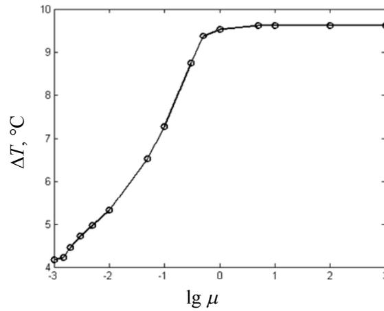
**Fig. 3.** Dependences of thermographic temperature difference on log of apparent milk viscosity as a result of numeric simulations.
