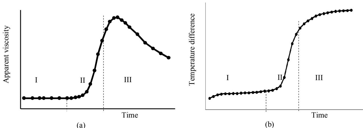
Fig. 1. Comparison of (a) a typical rheogram and (b) thermogram of rennet coagulation.
