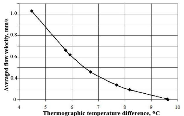
**Fig. 4.** Dependences of averaged flow velocity on thermographic temperature difference as a result of numeric simulations.
