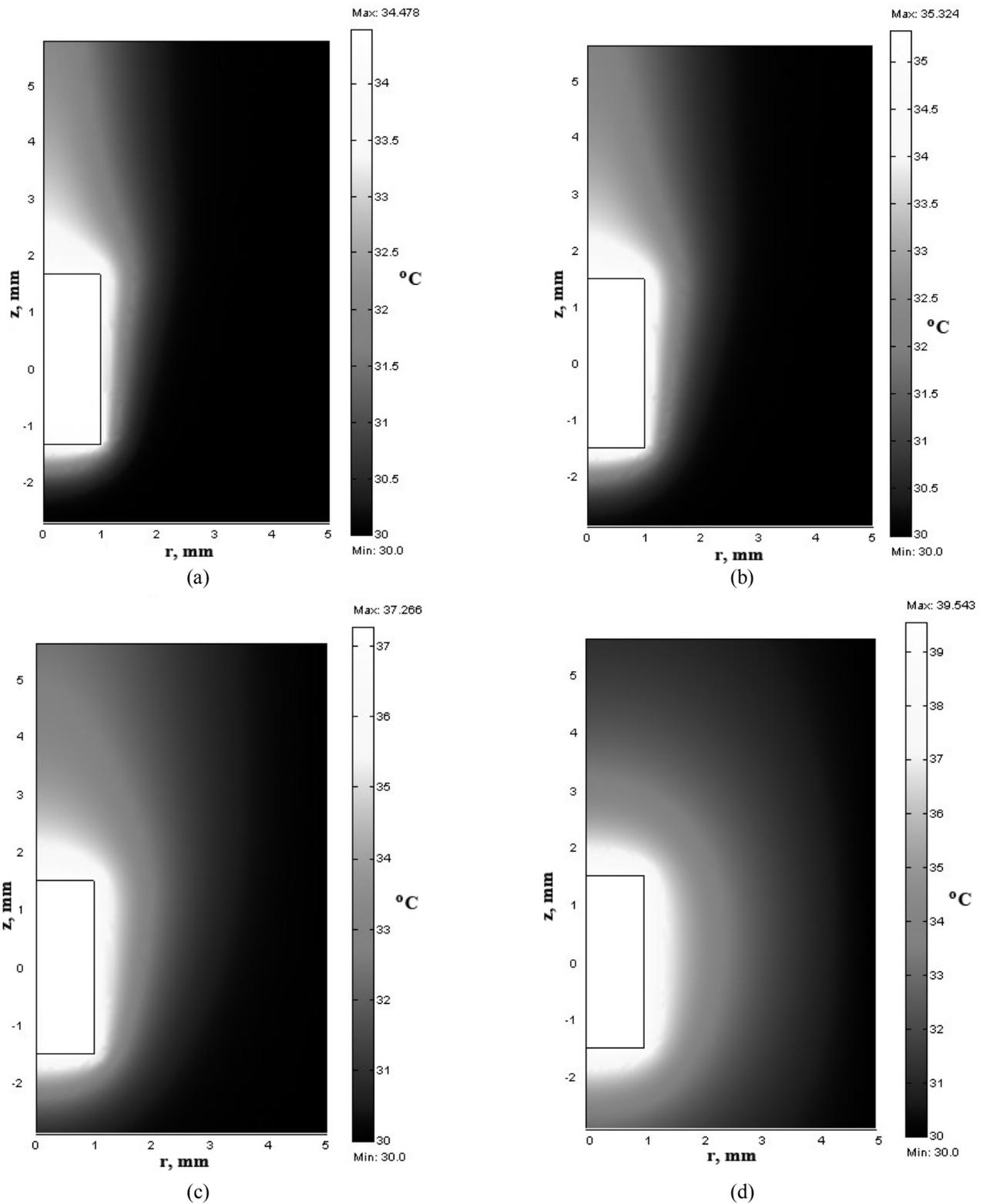
**Fig. 2.** Temperature distribution in milk with different apparent viscosities around the heated resistor. (a)  $\mu = 1.5 \cdot 10^{-3}$  Pa·s, (b)  $\mu = 1.0 \cdot 10^{-2}$  Pa·s, (c)  $\mu = 1.0 \cdot 10^{-1}$  Pa·s, and (d)  $\mu = 1.0$  Pa·s.
