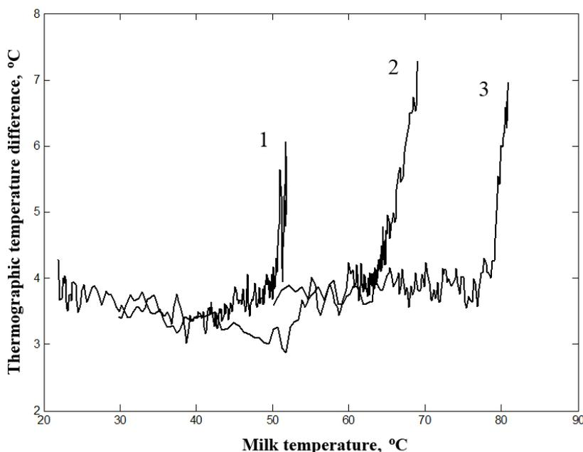
**Fig. 7.** Dependences of thermographic temperature difference on milk temperature for milk samples with different initial acidity: (1) pH = 5.6, (2) pH = 5.9, and (3) pH = 6.2.
