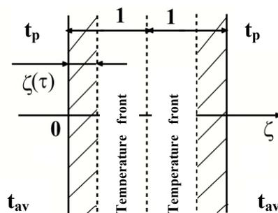
Fig. 4. Calculation diagram of the product at the further freezing stage.
