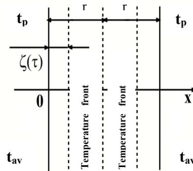
**Fig. 2.** Formation of the temperature front at the refrigeration stage.
