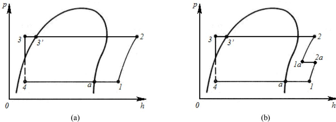
Fig. 1. Theoretical cycle of a refrigerating machine in the  $p$ - $h$  (pressure–enthalpy) coordinates: (a) one-stage compression cycle, (b) two-stage compression cycle.
