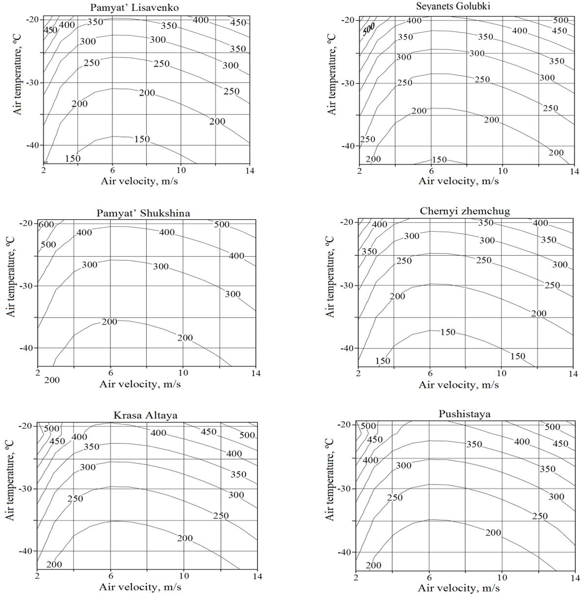
**Fig. 5.** Energy expenditures (kJ/kg) on the circulation of air in a fast freezer depending on the air velocity and temperature for the freezing of a kilogram of blackcurrant berries of studied varieties from the initial temperature of  $10^{\circ}\text{C}$  to the temperature of  $-18^{\circ}\text{C}$ .
