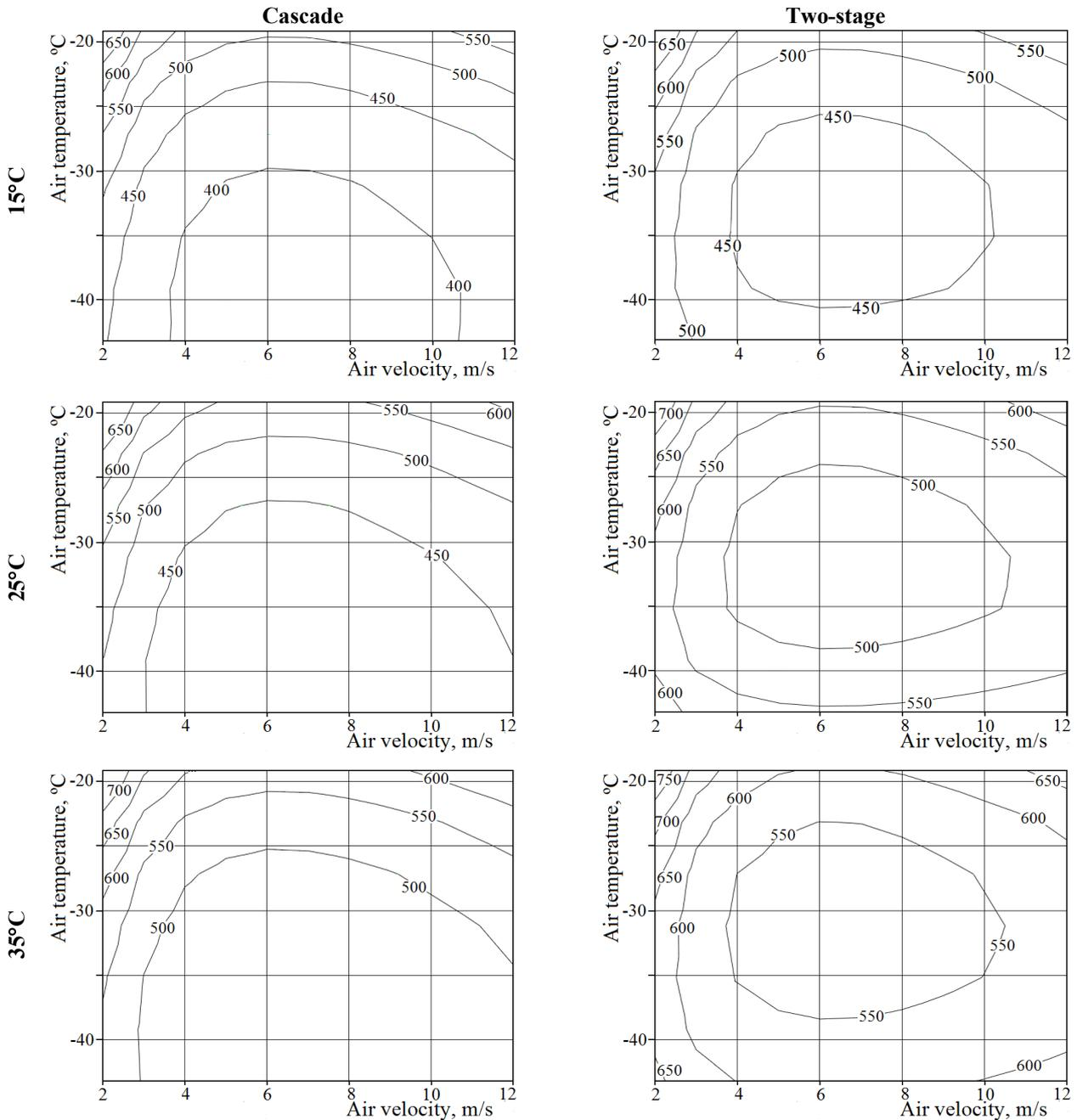
**Fig. 10.** Total energy expenditures (kJ/kg) on the freezing of Pamyat' Lisavenko blackcurrant berries in a fast freezer supplied with cold from cascade (R-23/R-22) and two-stage (R-22) refrigerating machines depending on the air temperature and velocity in a freezer and the ambient medium temperature.
