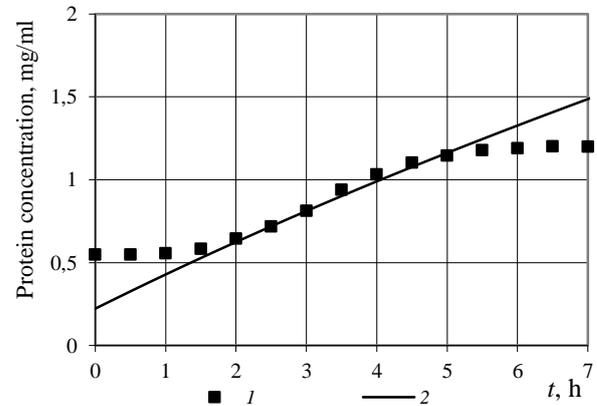
Fig. 4. Target biosynthesis product concentration versus cultivation duration: (1) experimental data, (2)  $P(t)$ .
