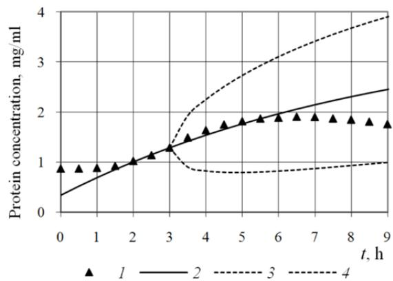
**Fig. 3.** Protein concentration versus cultivation duration: (1) experimental data, (2)  $M(t)$ , (3, 4)  $M(t) \pm \sqrt{D(t)}$ .
