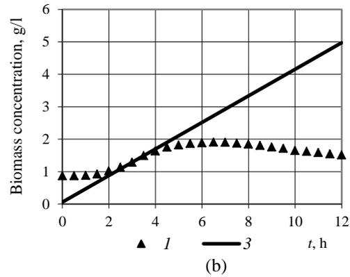
**Fig. 2.** Biomass concentration versus cultivation duration: (1) experimental data, (2) exponential growth curve  $M_0 \exp(\mu(t-t_0))$ , (3)  $M_0(t)$ .
