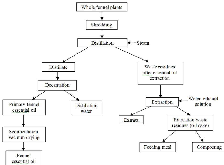
**Fig.4.** Scheme of the complex technology for the processing of fennel plants.
