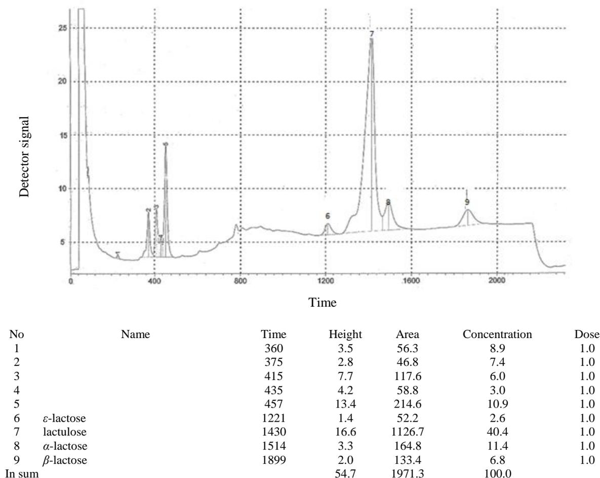
**Fig. 12.** GLC pattern of a lactulose solution with a mass fraction of solids of 40%.
