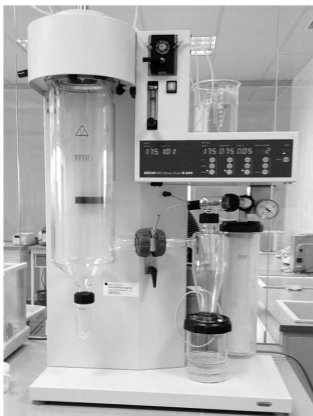
**Fig. 2.** Spray drying setup.
