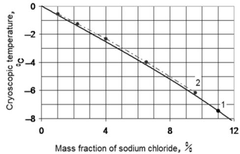
**Fig. 1.** Cryoscopic temperature of solution in function of sodium chloride concentration: 1, sodium chloride aqueous solution; 2, enzyme preparation.
