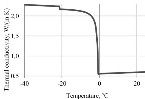
**Fig. 6.** Coefficient of thermal conductivity of L-phenylalanine ammonia-lyase enzyme preparation in function of temperature.
