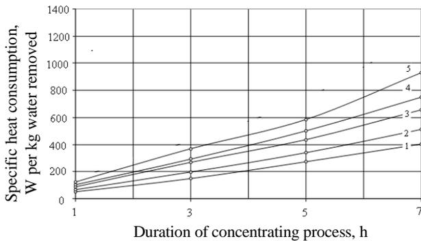
**Fig. 11.** Specific heat consumption during sublimation process of L-phenylalanine ammonia-lyase enzyme preparation in function of stabilization temperature of the dry layer: 1, 5°C; 2, 15°C; 3, 20°C; 4, 30°C; and 5, 40°C.
