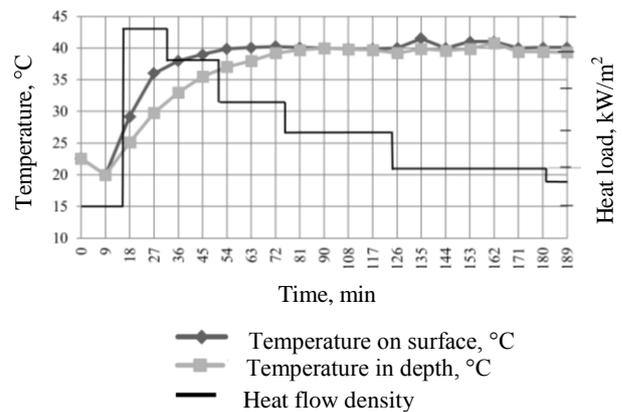
**Fig. 13.** Sublimation drying curves of the L-phenylalanine ammonia-lyase enzyme preparation at heat load of 9.2 kW/m<sup>2</sup>.
