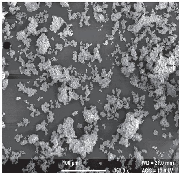
**Figure 8** SEM image of the activated charcoal
