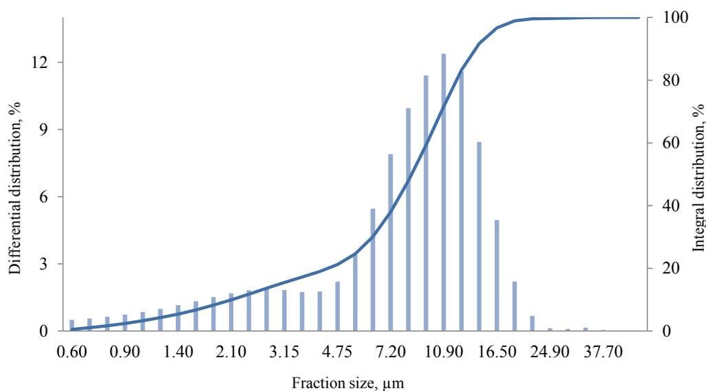
**Figure 8** Granulometric composition of the hydrolysate after spray-drying
