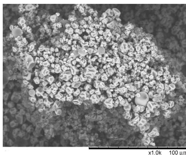
**Figure 7** Scanning electron microscopy of the hydrolysate after spray-drying
