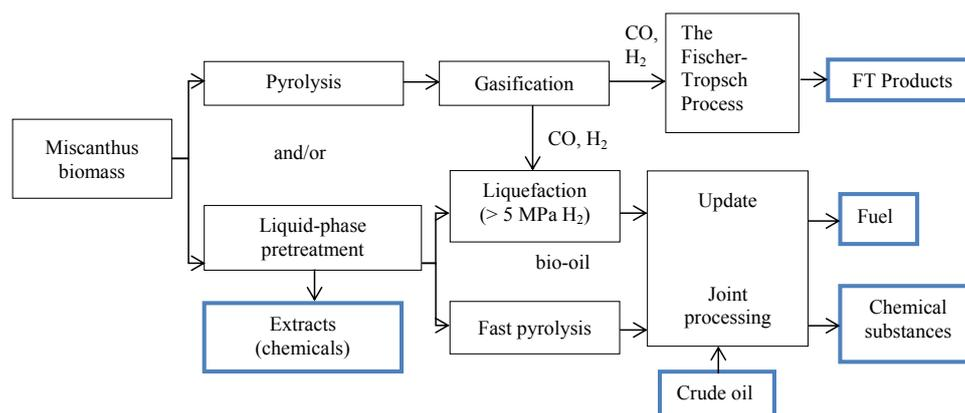
**Figure 4** Simplified scheme of fuel and chemicals production
