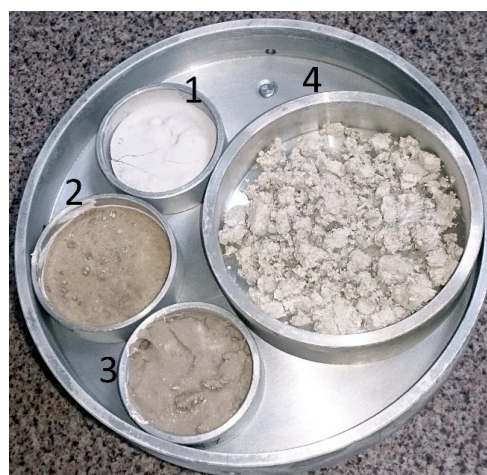
Figure 4 Frozen fractionation products before freeze drying: 1–4 are numbers of corresponding fractions
