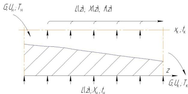
Fig. 8. Diagramme of interaction of the coolant flow and the fluidised bed of the dryable product moving along the cylindrical surface.
