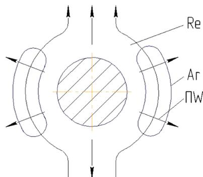
**Fig. 6.** Motion modes during continuous drying: Re – forced; Ar – free natural; PW – diffusive.
