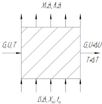
Fig. 9. Material flows in the moving element of the wet solids.
