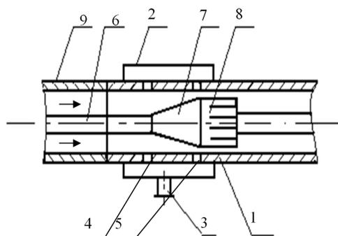
**Fig. 4. Membrane module with devices for the withdrawal of the concentrate and the mechanical cleaning of a membrane: (1) housing, (2) shell, (3) fitting, (4), (5) annular slots, (6) guiding rod, (7) cone, (8) cleaning device, (9) tubular ceramic membrane.**
