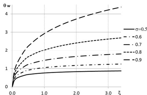
**Fig. 6. Effect of the membrane selectivity on the distribution of surface concentrations.**
