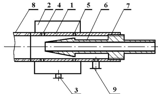
**Fig. 3. Device for the separation of the near-membrane layer: (1) housing, (2) shell, (3), (9) fittings, (4), (5) slots, (6) rod, (7) thread, (8) tubular membrane.**
