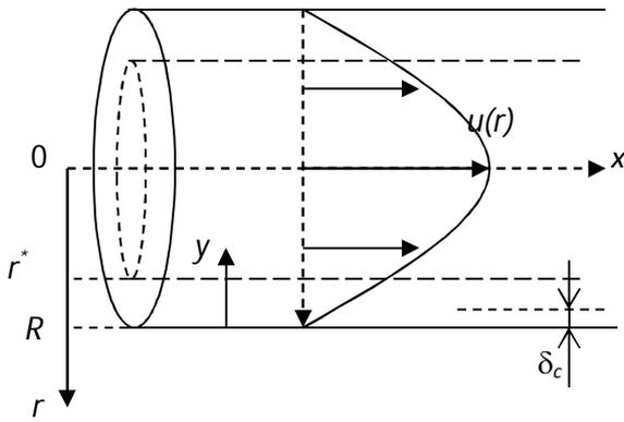
**Fig. 2. Separation of the flow of a solution in a tubular membrane.**
