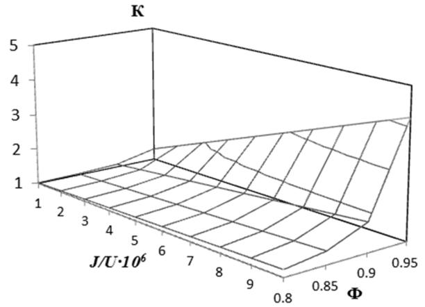
Fig. 7. Concentration coefficient of an ideal membrane for the separation of the near-wall flow part.
