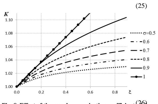
Fig. 8. Effect of the membrane rejection coefficient of the efficiency of concentrating.
