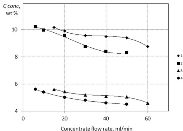
**Fig. 10.** Total solids content in the concentrate: (1), (3) on the membrane with 200-nm pores, (2), (4) on the membrane with 20-nm pores, (1), (2) the medium is skim milk, and (3), (4) the medium is dairy whey ( $p = 0.15$  MPa,  $t = 20^\circ\text{C}$ ,  $Re \approx 500$ ).
