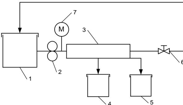
**Fig. 1. Laboratory bench scheme: (1) initial solution vessel, (2) pump, (3) membrane module, (4) permeate collection vessel, (5) withdrawn concentrate collection vessel, (6) valve, (7) manometer.**
